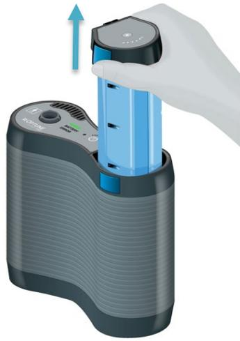
Recharge the batteries in the charger (see Section 15) for four to five hours. The batteries will stay charged if they are off the charger for a short time (hours, but not days). For this reason, keep the extra batteries in the charger at all times, if possible.
