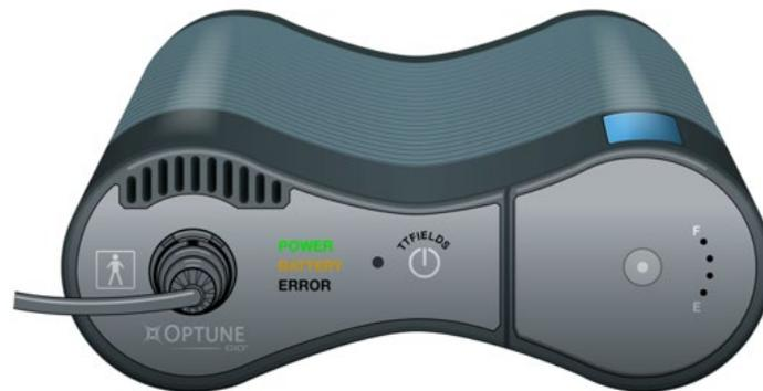
When your battery runs out (after about 2–3 hours), the notification signal will beep, and the TTFIELDS treatment will stop. When this happens the "Battery" indicator will turn yellow and red Error light will light up. This notification signal sound is the same sound the device makes for an error. However, in this case both the yellow "Battery" and red "Error" indicators will light up instead of just the red light.
