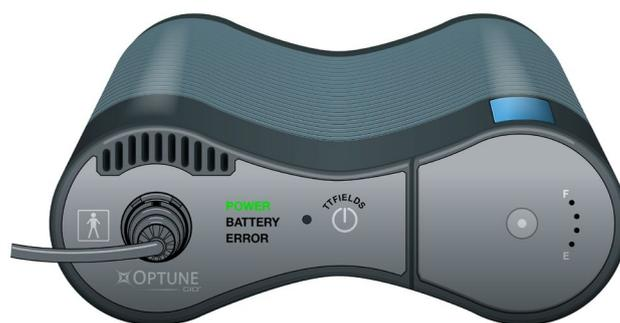
If a charged battery is installed and there is no power supply plugged in, the "Battery" indicator will also light up green.
